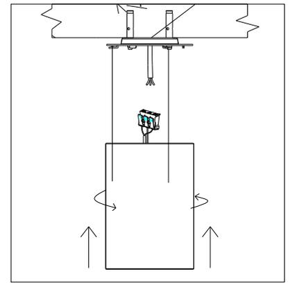
3. Place driver into metal housing. Connect mains with the driver. Install the metal housing onto fixing ring and lock it.
