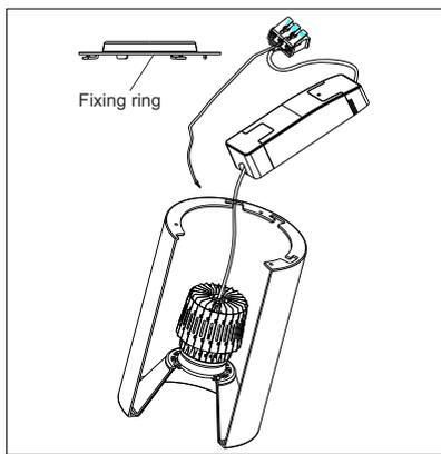
1. Remove front ring from luminaire. Screw in the luminaire into metal case. Connect luminaire to driver.
