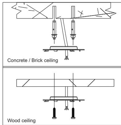
2. Fix the mounting ring to ceiling with corresponding screws. Put the mains line through fixing ring.
