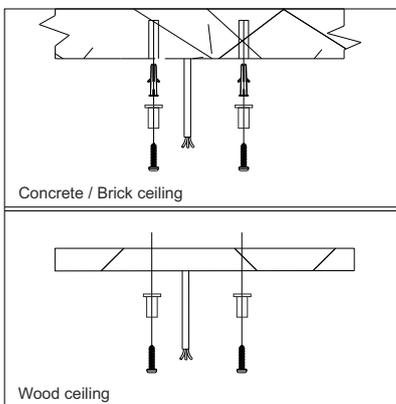
1. Install the rope suspension kit with corresponding screws to the ceiling.
