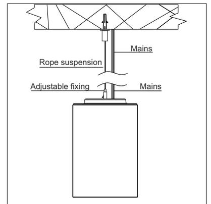
3. Connect the mains to driver. Place the luminaire at desired height and shorten rope accordingly.
